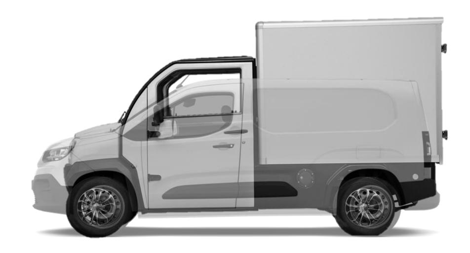
As an L7e category platform, it weighs about half as much as an internal combustion engine (ICE) compact van with a similar payload volume.
